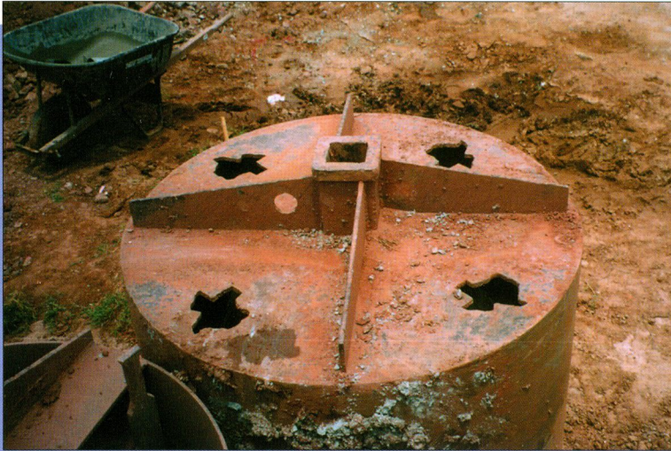
Texas Shafts signature core barrel used for sandstone removal.
